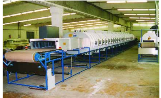
Mikrowellen-Banddurchlauf-Trockner Microwave continuous belt dryer 25 m / 70 kW
