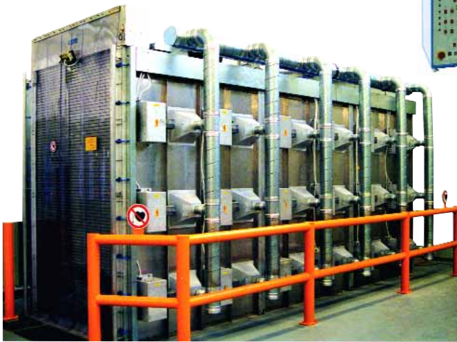
Mikrowellen-Kammertrockner Microwave chamber dryer 21 m 3 / 30 kW
