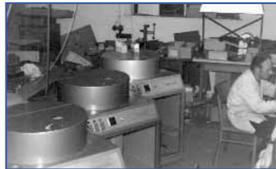
Induction casting units, 1970
